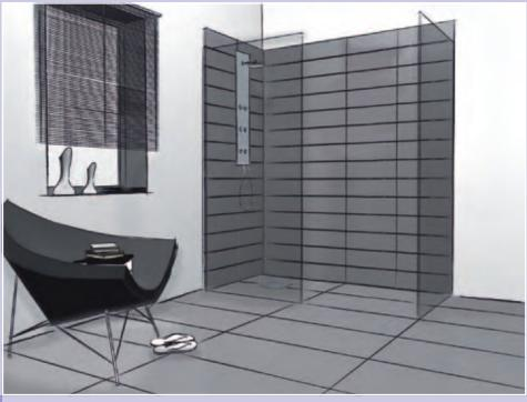
Open and barrier-free: The glass partition walls are installed lengthwise and across in such a way that water cannot spray out into the room, even though there is no door. And the walkin access creates a lovely modern shower with no risk of stumbling.
