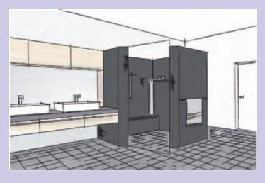
Tiles can be laid straight onto JACKOBOARD Aqua. All types and sizes of tiles can be used in principle. Special requirements only apply to showers that must offer wheelchair access or to mosaic tiles < 25 mm.
